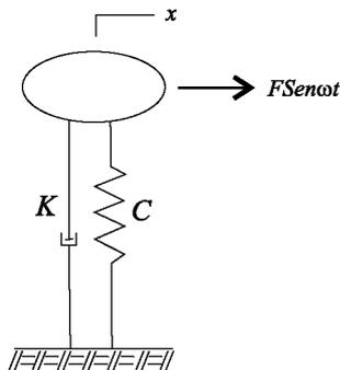
$$\ddot{x} + 2b\omega_1\dot{x} + \omega_1^2 x = F \text{ Sen } \omega t$$
