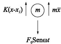
$$m\ddot{x} + K(x - x_1) = F_0 \text{ Sen } \omega t \dots\dots(1)$$
