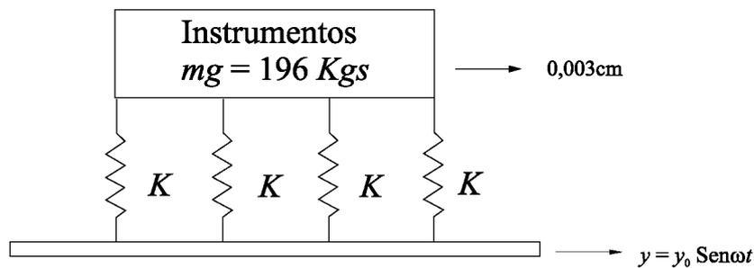
$$\frac{A}{y_0} = \frac{\sqrt{1 + \left(2b \frac{\omega}{\omega_1}\right)^2}}{\sqrt{\left[1 - \left(\frac{\omega}{\omega_1}\right)^2\right]^2 + \left(2b \frac{\omega}{\omega_1}\right)^2}}$$
