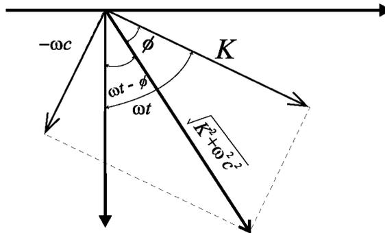
$$\phi = \text{arctg} \left( -\frac{\omega c}{K} \right)$$
