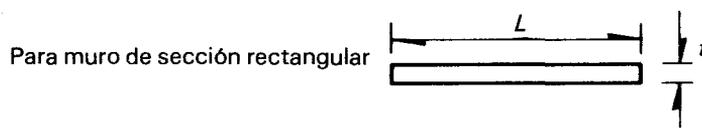
$$\begin{aligned} A &= tL \\ I &= \frac{tL^3}{12} = \frac{AL^2}{12} \quad G = \frac{E}{2(1+\nu)} = 0.4E \quad \alpha = 1.2 \\ \frac{\Delta_F}{\Delta_v} &= \frac{VH^3}{3EI} \frac{GA}{\alpha VH} = \frac{H^2 0.4 EA}{3E AL^2 \alpha} = 1.33 \left(\frac{H}{L}\right)^2 \end{aligned}$$
